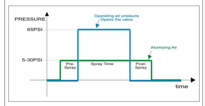
FIG. 7: Timing Diagram
