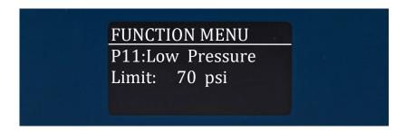
Fig. 18: Low Pressure Limit
