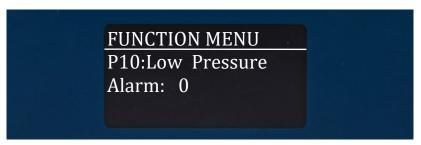
Fig. 14: Low Pressure Alarm
