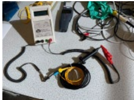
Figure 1. Measurement of end-to-end resistance of dispenser assembly
