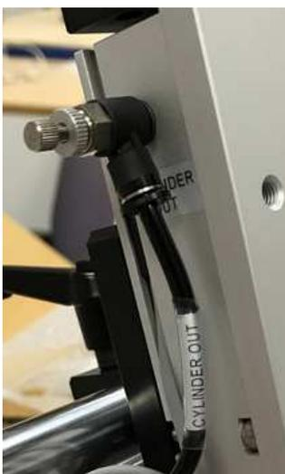
Cylinder out flow regulator, showing locking nut and adjustable knob for flow rate.
