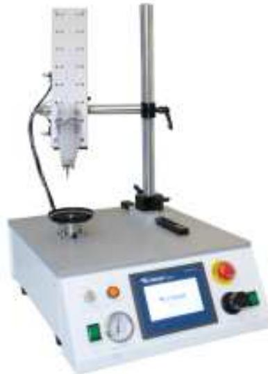
The Z-axis tilt is easily adjusted to dispense either on a vertical wall within a cylindrical part or on an outside wall. The system is fully programmable to control dispense delay, degree of rotation and wait period before cycling using the intuitive user friendly HMI display.
