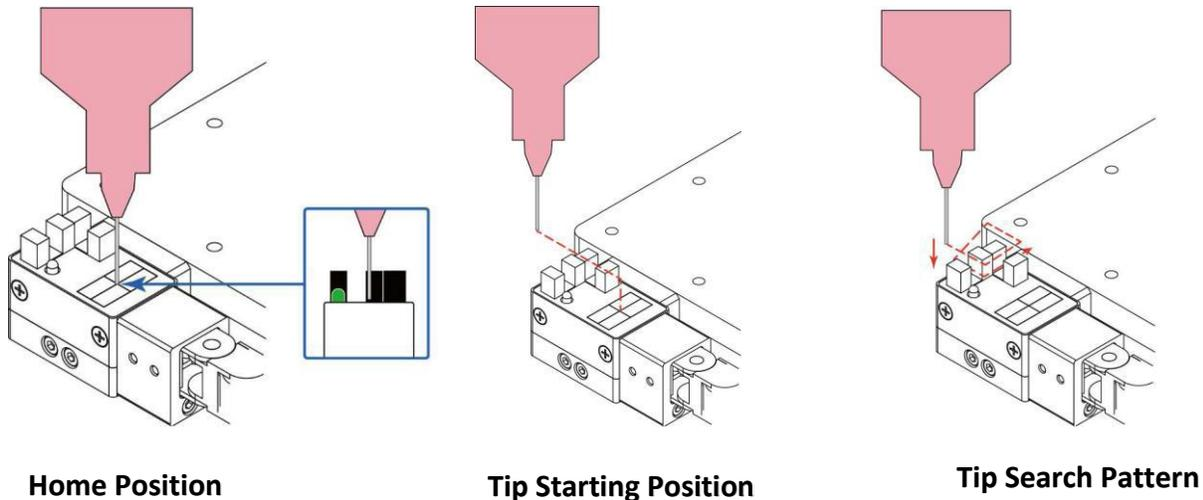
The above images show the movements and positions the Tip Alignment Device makes when it is correcting for offsets. Home Position, Tip Starting Position and the Tip Search Pattern are all shown above.
