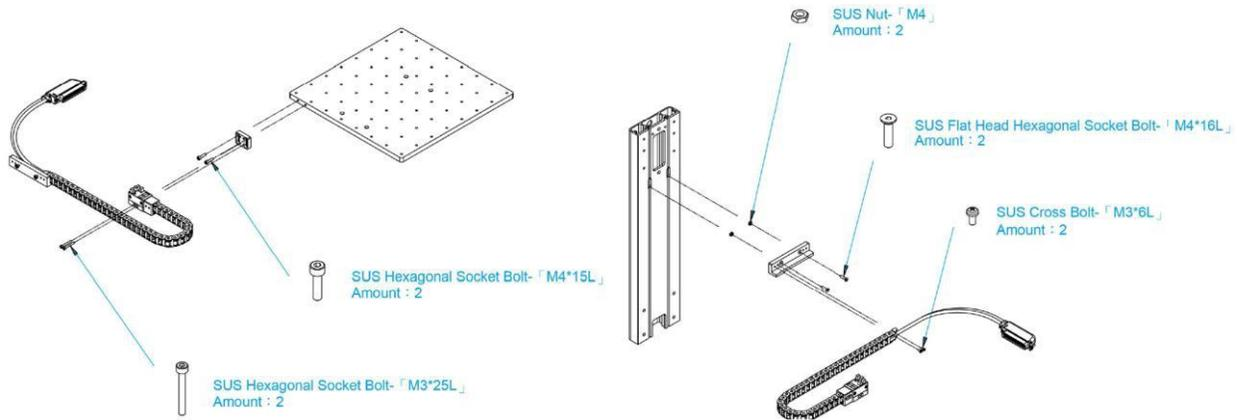
Shown above is the device connection to the robot work plate as well as a way to secure it to the robot side. During installation, please try and correctly level the device as any offsets can affect the tip correcting functionality.
