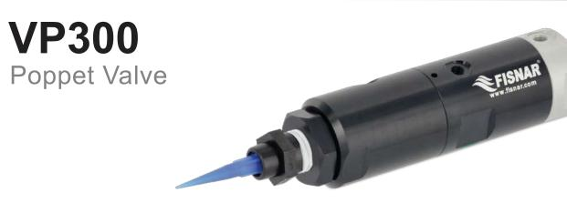
The VP300 is a multipurpose, poppet-type pneumatic valve designed for dispensing low to mid-high viscosity materials, such as silicone, RTV, epoxy, rubber adhesive, grease, liquids containing filler, etc. A diaphragm located between driving parts and wetted parts increases the valve life and reduces valve maintenance.
