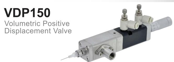
The VDP150 plunger pump is a pneumatically operated positive displacement valve designed for dispensing constant volume shots of low to medium viscosity materials within 1%. The VDP150 has two integral check valves to control the flow of material.
