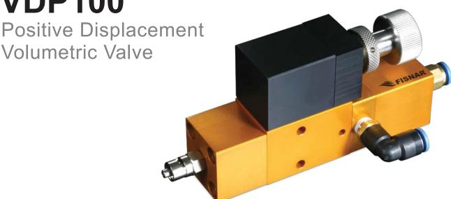
The VDP100 is an adjustable pneumatically operated positive displacement valve designed for dispensing constant volume shots of low to medium viscosity materials within 1%, such as oil and grease. The VDP100 valve has a range up to 0.9cc.
