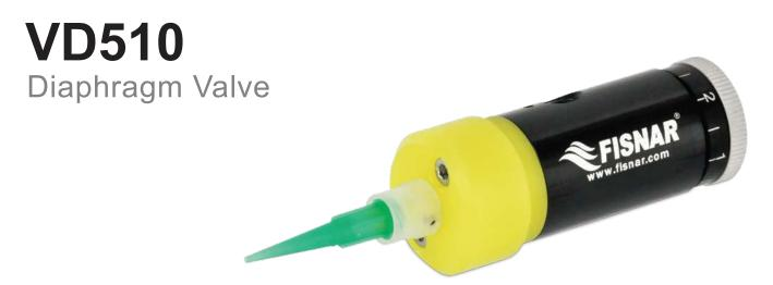
The VD510 is a diaphragm valve designed for precise flow control of low to medium viscosity materials. The diaphragm separates the wetted parts from the moving parts and, therefore, the valve is ideal for dispensing cyanoacrylates, reagents, electrolytes, glues, solvents, paints, alcohol and other volatile substances.
