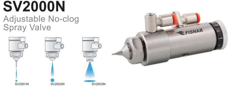
Fisnar spray valves provide close tolerance spray dispensing of fluids up to 1000 cps, including urethanes, flux and paints. The material is fed from a pressure reservoir. Each valve is actuated by air pressure sequenced by a controller. The operating air pressure opens a needle valve allowing material to flow; a separate air line creates pressure in the air cap, atomizing the fluid.
