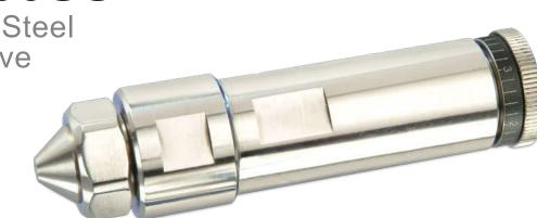
The SV1000SS spray valve provides close tolerance spray dispensing of fluids of up to 1000 cps. The SV1000SS is constructed of stainless steel to prevent corrosion from volatile materials. With a spray angle of 12 degrees and an operating frequency of 200 cycles/min, the SV1000SS is designed for spraying flux, urethane, paint, lubricants, and for coating and conformal coating and marking applications.
