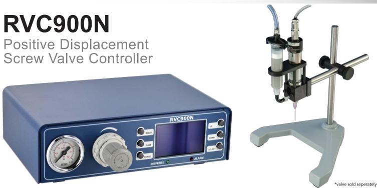
The RVC900N controls the PDV-1000 series of auger valves and the model RV5000DPM disposable cartridge auger valve. The controller is programmable for timed shots from a minimum of 0.01 seconds. Motor speed output is maintained and kept constant, compensating for any change in material viscosity.
