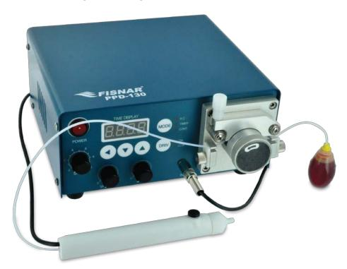
Peristaltic pump dispensers transfer low viscosity liquids by pressure displacement applied to a turning rotor against a tube carrying material. Usually these pumps are chosen because the liquids are hazardous or difficult to work with and it is advisable to limit operator contact. Another reason is that peristaltic pumps are air free.
