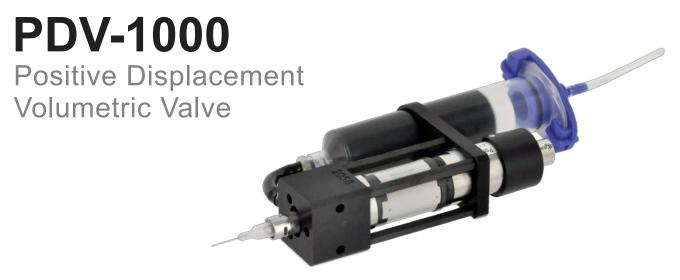
The PDV-1000 series of precision auger valves is suitable for all medium to high viscosity paste, epoxy, solder paste and other filled material. Capable of dispensing a minimum shot size of 0.020" (0.508mm), the PDV-1000 uses an auger servo-motor driven screw.
