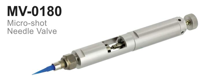
Designed for precision dispensing of all types of fluids from micro shots to moderate sized beads and dots. Its lightweight pencil-type grip makes the valve suitable for either hand-held or automatic applications. Shot sizes may be fine tuned by turning the adjustment knob at the top.
