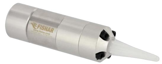
The 790HP-LF series high-pressure dispense valve is an economic solution when dispensing high viscosity materials such as silicones, RTV, sealant and grease. The 790HP-LF provides a snap-release shut off after dispensing, resulting in a suck-back at the fluid outlet, preventing any drip or post extrusion.
